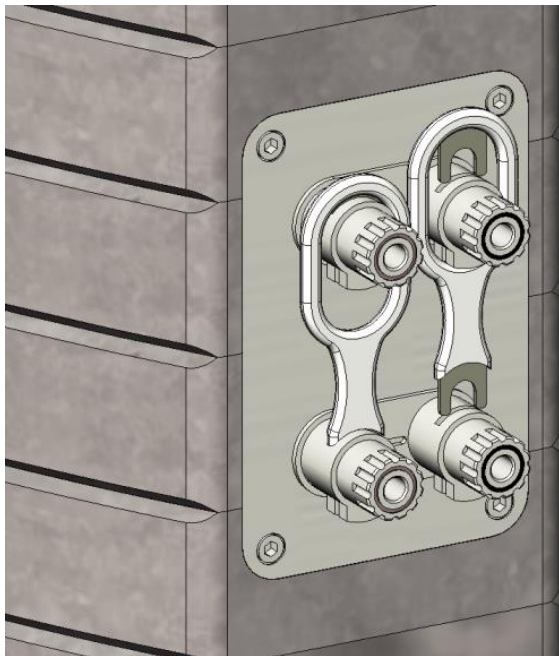
Figure 4: Remove terminal jumpers/bridges if using bi-wire connection.
